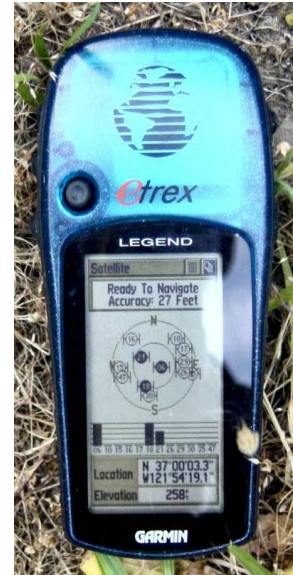
Three strong satellites signals displayed on Garmin eTrex Legend
