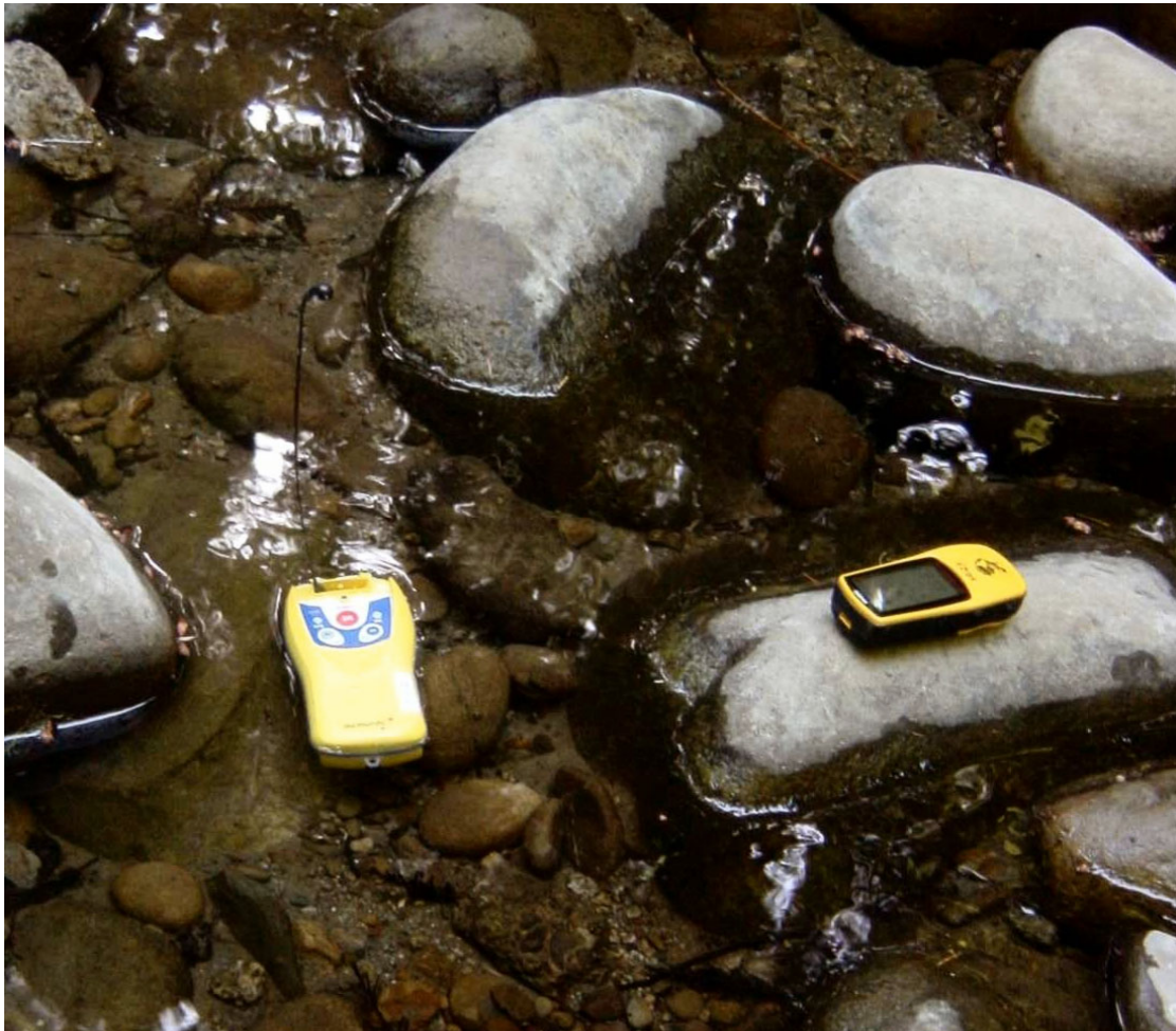
Fastfind Plus PLB floating in Aptos creek at bottom of ravine. Only one satellite is displayed on the adjacent Garmin eTrex
