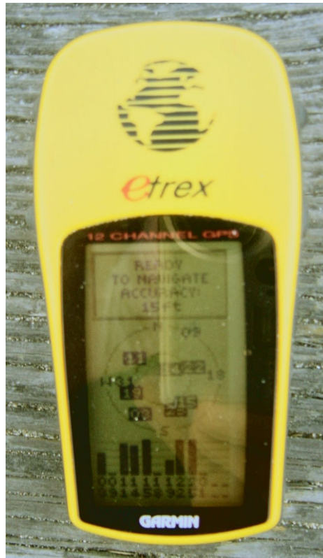
Garmin eTrex on wooden pier, showing 7 satellites visible.
